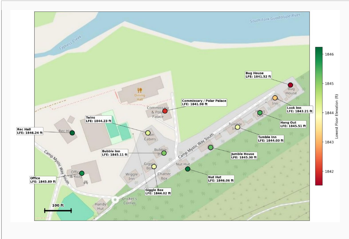
Figure A-2. Map of selected buildings at Camp Mystic Guadalupe River, with elevations.
